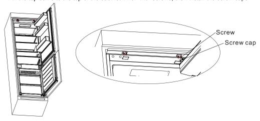
Open the lower door of cabinet the maximum angle, and open the lower door of the refrigerator to the
