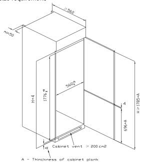
• Push the refrigerator into the cabinet and adjust it to make sure the edge fold of top baffle completely touch the top edge of the cabinet, and the limit hook of supporting leg completely touch the bottom edge of the cabinet.
